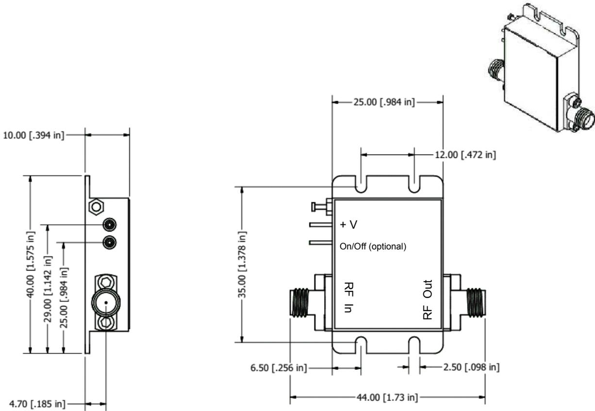
Field replaceable SMA Connectors, Removable Ground slug
