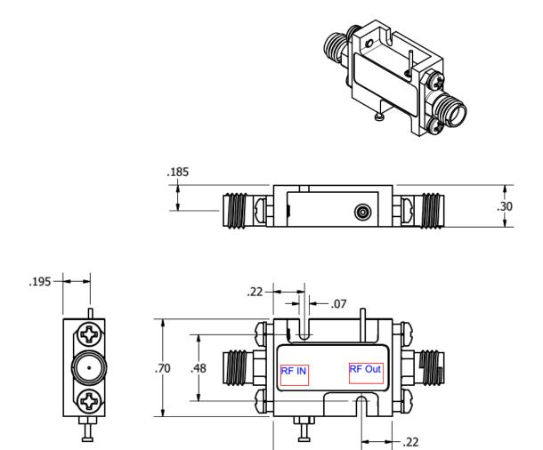
Amplifier must be properly attached for heat dissipation Removeable SMA and Ground slug
