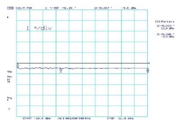
AM/PM Phase Change with Pin Sweep from -10 to +11 dBm @ 1 GHz
