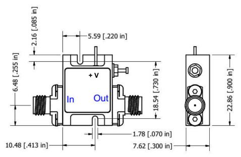
Field replaceable SMA Connectors, Removable Ground Slug
