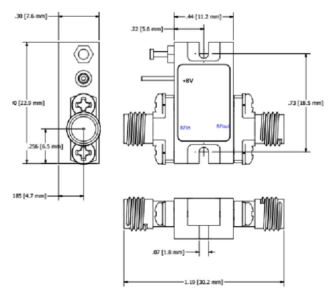
SMA Connectors and ground slug are field replaceable Housing: Aluminum Gold over Nickel plated
