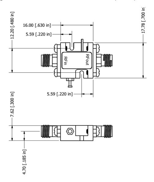
Housing: Aluminum Gold over Nickel plated Removable SMA and Ground Slug
