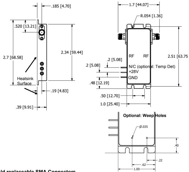
Field replaceable SMA Connectors Housing Material Aluminum, Nickel Plated
