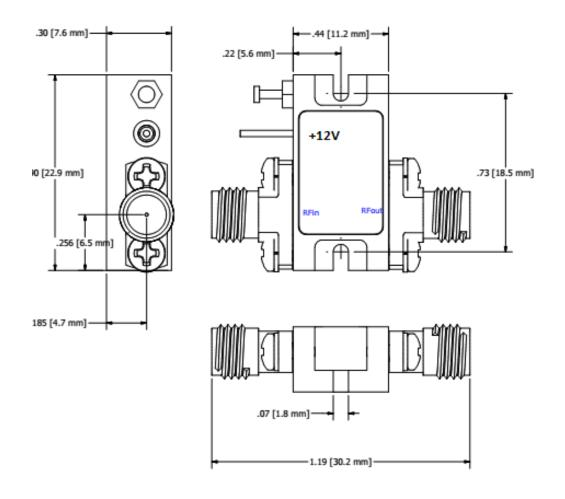
Housing: Aluminum Gold over Nickel plated Removable SMA and Ground Slug
