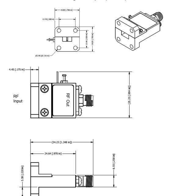
Field replaceable 2.92mm SMA Connector at output
