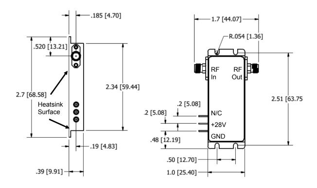
Field replaceable SMA Connectors Housing Material Aluminum, Nickel Plated
