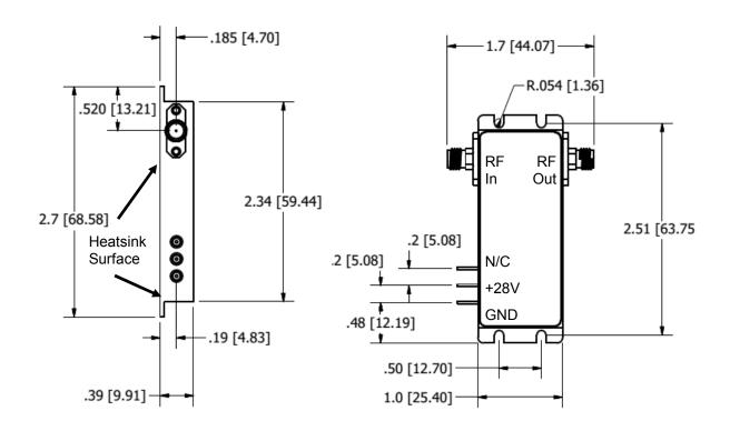
Field replaceable SMA Connectors Housing Material Aluminum, Nickel Plated
