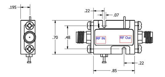
Amplifier must be properly attached for heat dissipation Removeable SMA and Ground slug
