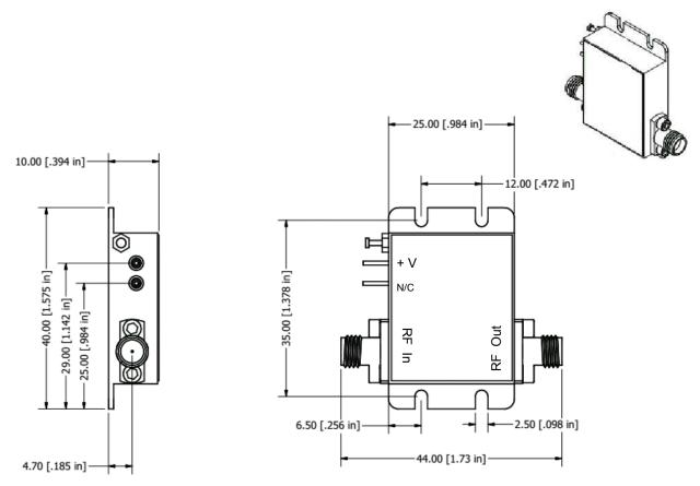
Field replaceable SMA Connectors, Removable Ground slug
