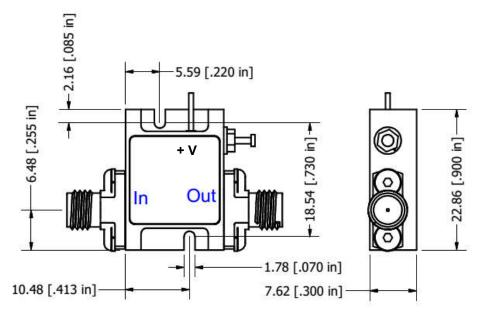
Field replaceable SMA Connectors, Removable Ground Slug
