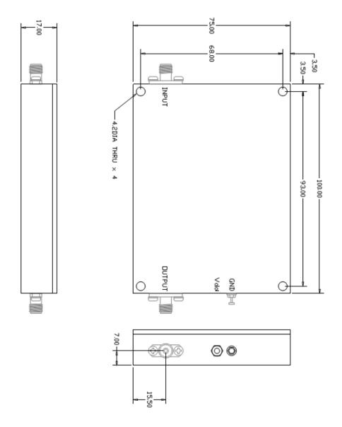
Note: The unit must be attached to proper heat sink with thermal interface material (Thermal Pad or Thermal Grease)
