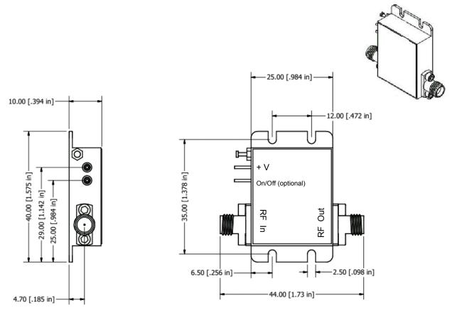
Field replaceable SMA Connectors
