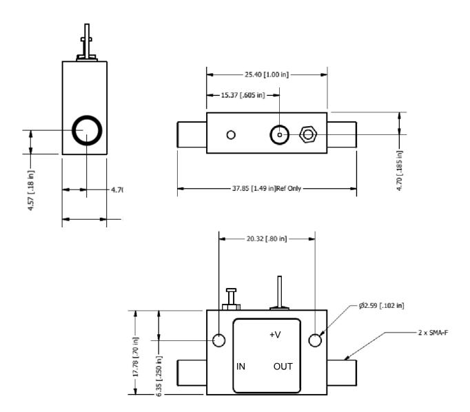
Housing: Aluminum Gold over Nickel plated Removable SMA and Ground Slug
