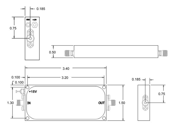
Note: The unit must be attached to proper heat sink with thermal interface material (Thermal Pad or Thermal Grease)
