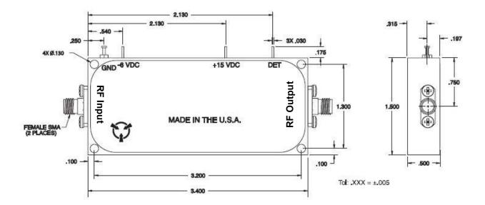
Note: The unit must be attached to proper heat sink with thermal interface material
