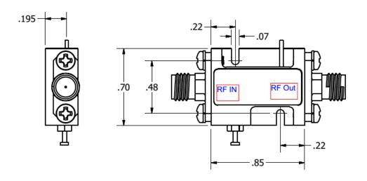
Amplifier must be attached properly to dissipate heat Removeable SMA and Ground slug
