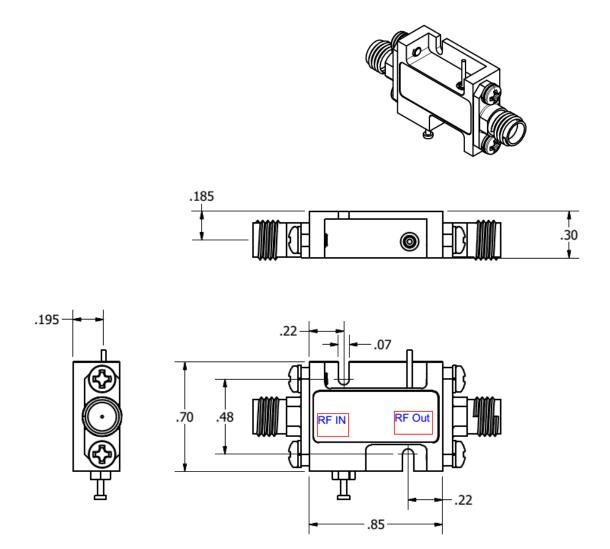
Amplifier must be properly attached for heat dissipation Removeable SMA and Ground slug
