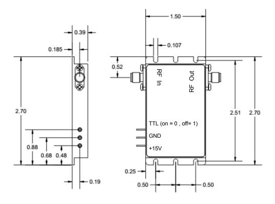
Field replaceable SMA Connectors TTL on/off optional
