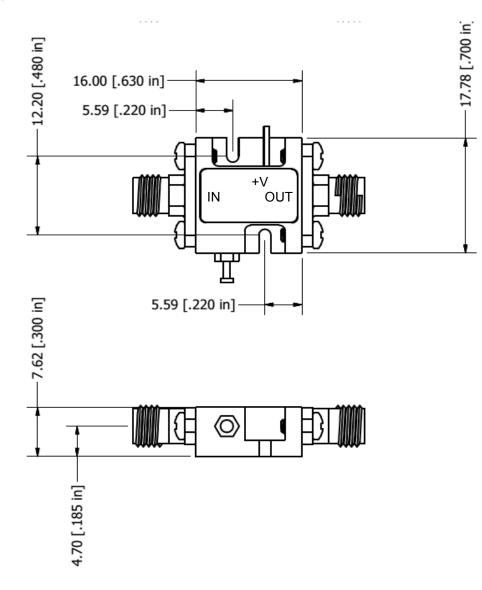
Housing: Aluminum Gold over Nickel plated Removable SMA and Ground Slug
