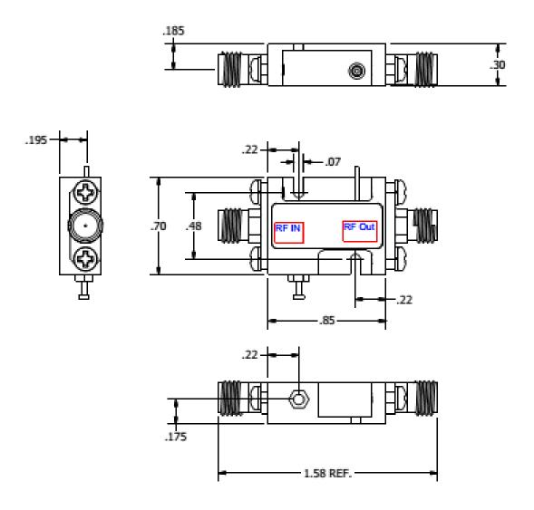
Housing: Aluminum Gold over Nickel plated Removable SMA and Ground Slug
