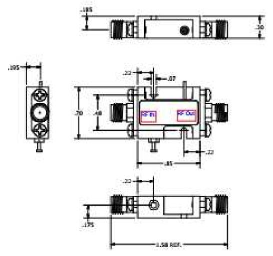
Ground Slug is 0.180 long from base SMA Connectors and Ground Slug are removeable
