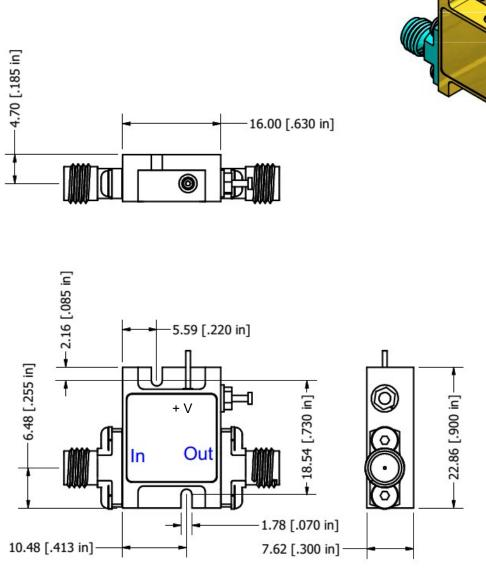
Field replaceable SMA Connectors Housing material: Aluminum 6061-T6 Plating: Gold over Nickel Note: The unit must be attached to proper heat sink
